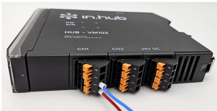
Connecting a “PCB Piezotronic” vibration sensor to the HUB-VM102 (with wire-end ferrules in this example)
