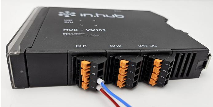
Connecting cable of a PCB Piezotronics vibration sensor at the HUB-VM102
