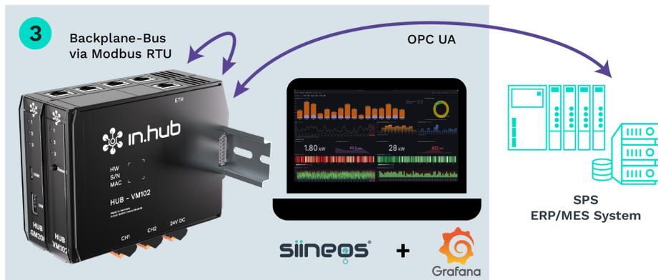
1. Install one device or more on the backplane bus of the master gateway, which is already located on the DIN rail in the control cabinet.
