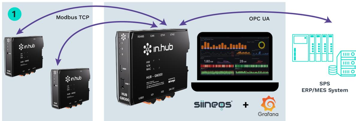
1. Install one device or more on the DIN rail in the control cabinet.
