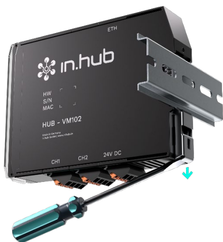
Fig. 5: Removing the HUB-VM102 from the DIN rail
