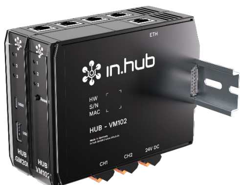
Fig. 4: Master gateway HUB-GM200 with a HUB-VM102
