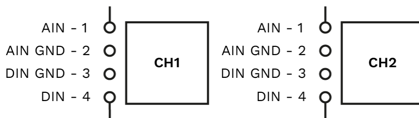
Fig. 6: Schematic drawing of the CH1 and CH2 interface
