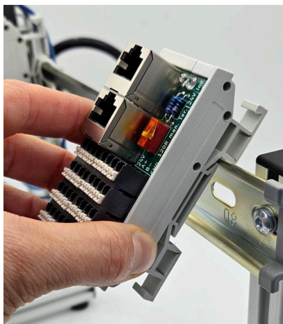
Mounting the HUB-RTU
