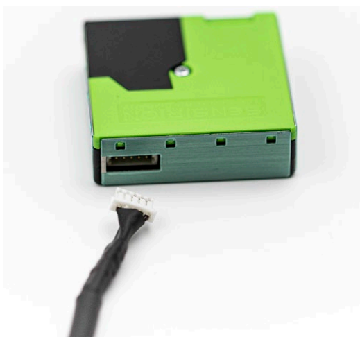
Fig. 3: Connection of sensor cable to particle sensor
