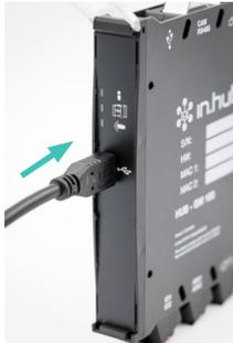
Connect your PC with the gateway using a micro USB cable.
