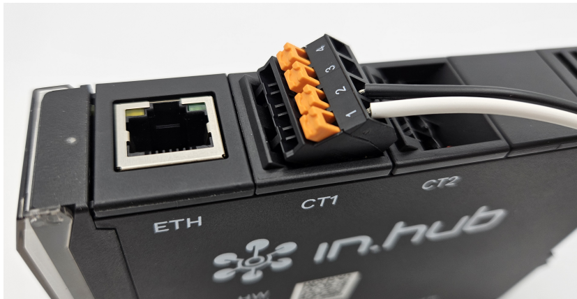
Connection of a SENS-CUR current sensor to the HUB-EN200
