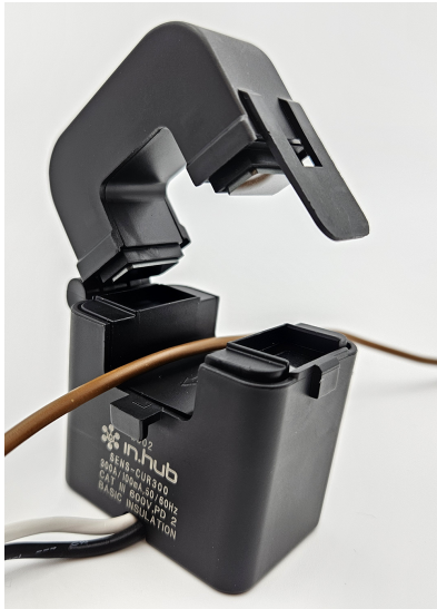
Opened SENS-CUR current sensor with live cable next to a schematic diagram for connecting the current sensor
