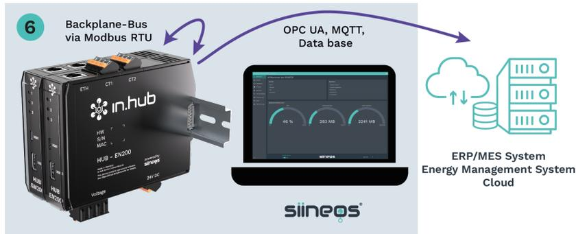
1. Install the device on the backplane bus of the master gateway, which is already located on the DIN rail in the control cabinet.
