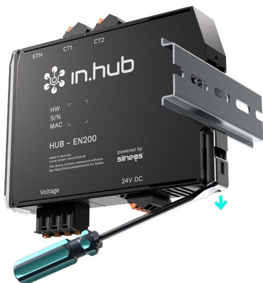
Removing the HUB-EN200 from the DIN rail
